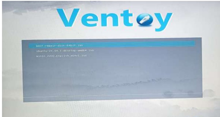
Figure 5.4: Screenshot of Multi-OS Bootable USB created using Ventoy.ISO files for Boot-Repair, Ubuntu 24.04 and Windows 10
