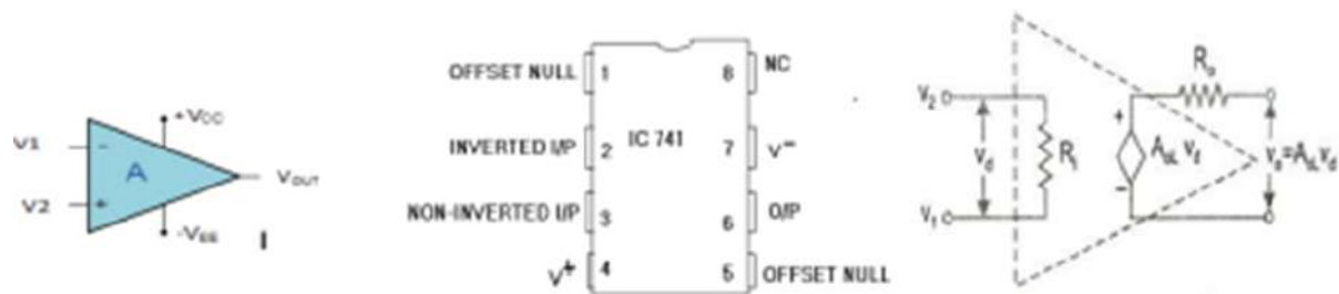
Op-amp symbol, Op-amp pinout, and equivalent circuit
